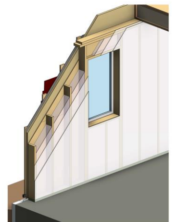
3) Energy efficient prefabricated wood panel
